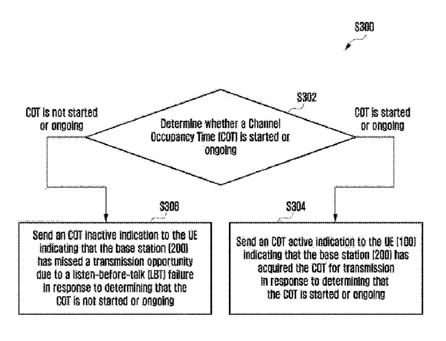
includes indicating, by the UE, about the acquired COT to a MAC layer from a physical layer. The physical layer indicates one of the base station has acquired the COT for transmission and the base station has missed a transmission opportunity due to a LBT failure.
