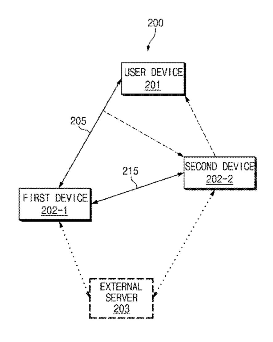
information is used by the second external electronic device to monitor the first link, negotiate timing for transmitting a response message with the second external electronic device, receive a data packet from the first external electronic device, and transmit a response message to the first external electronic device in response to the data packet based on the negotiated timing.
