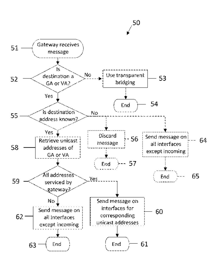
addressed by the retrieved unicast addresses are serviced by the gateway device, sending the received message on all network interfaces except for the network interface over which the message was received.
