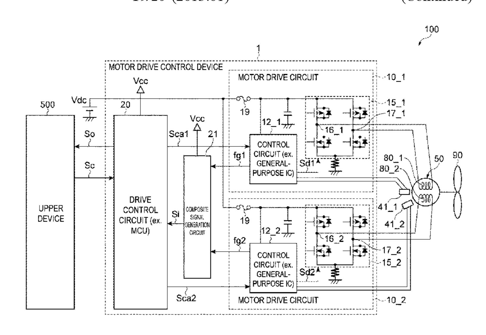
drive circuits. The FG signals output from the motor drive circuits have a phase difference from each other.
