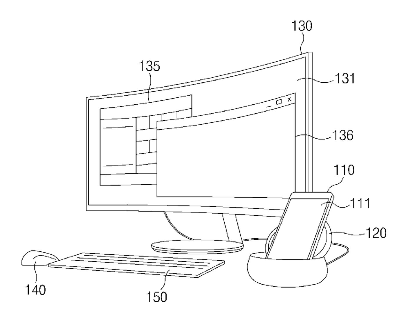
tronic device, provide at least a portion of the display for use as a pointing device.
