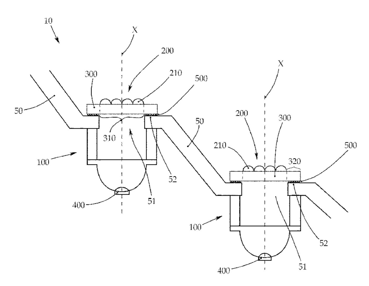
(300) comprises an edge section (320) surrounding the optically active section (310) and projecting in a partially planar extension of the optically active section (310), wherein the edge section (320) is attached to the support frame (50) at least in sections by means of an adhesive (500).
