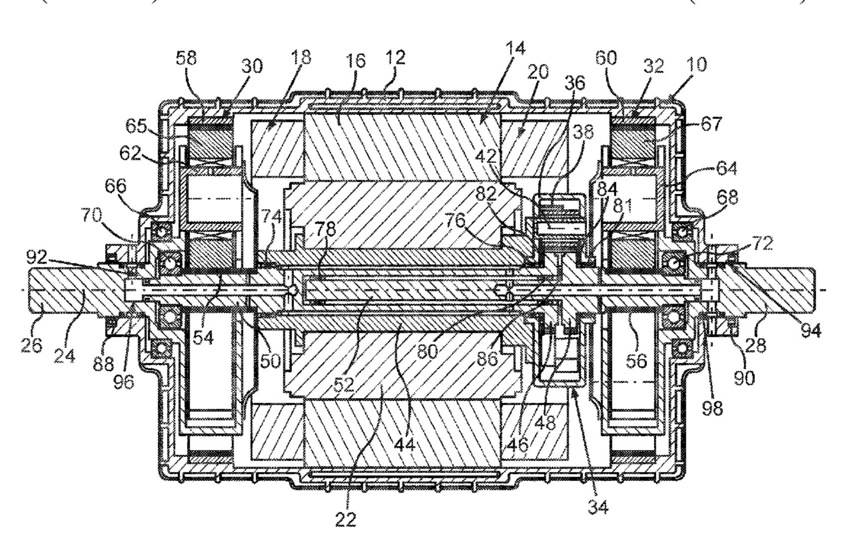
differential shaft. The further bearings are arranged spaced apart from one another at least at a distance of twice an average bearing diameter.
