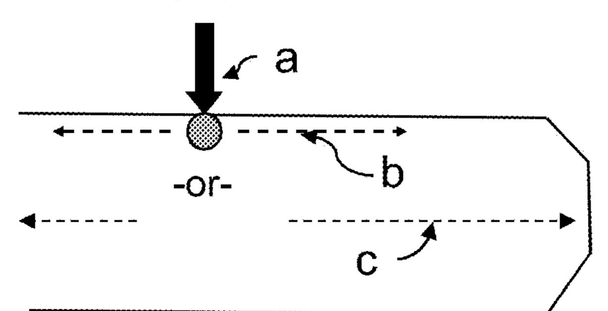
fracture propagates from bending on top (or from Center Tension)
