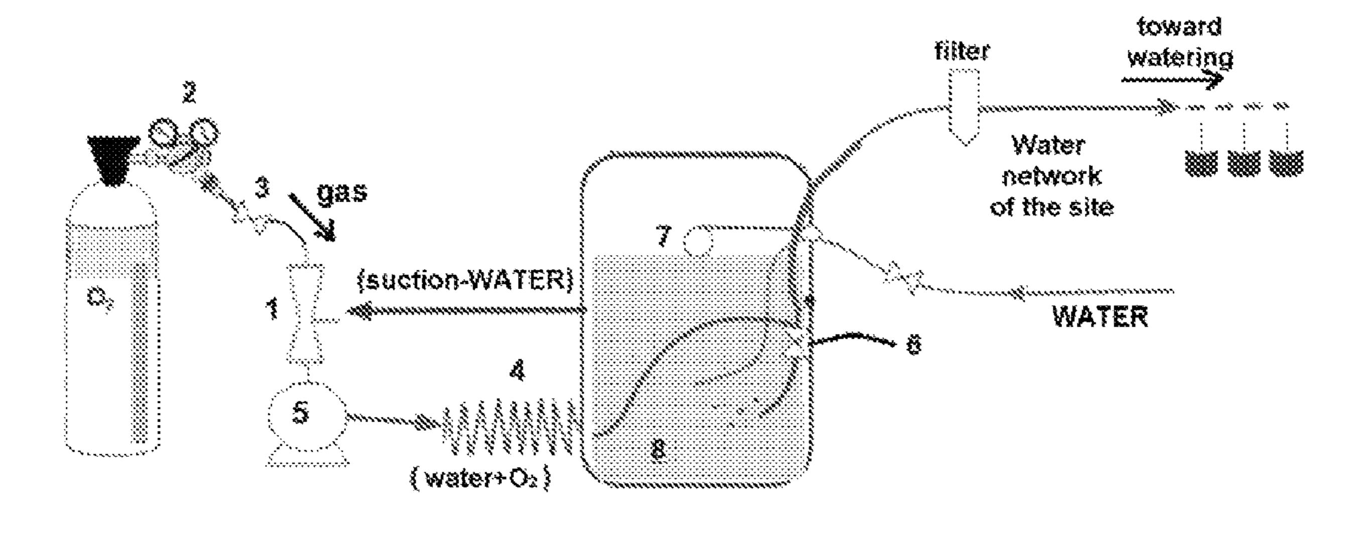
to direct the water entirely to the animals' watering or partially to the animals' watering and partially back to the water tank. A method for rearing animals includes boosting water with dissolved oxygen up to saturation for animals' watering.
