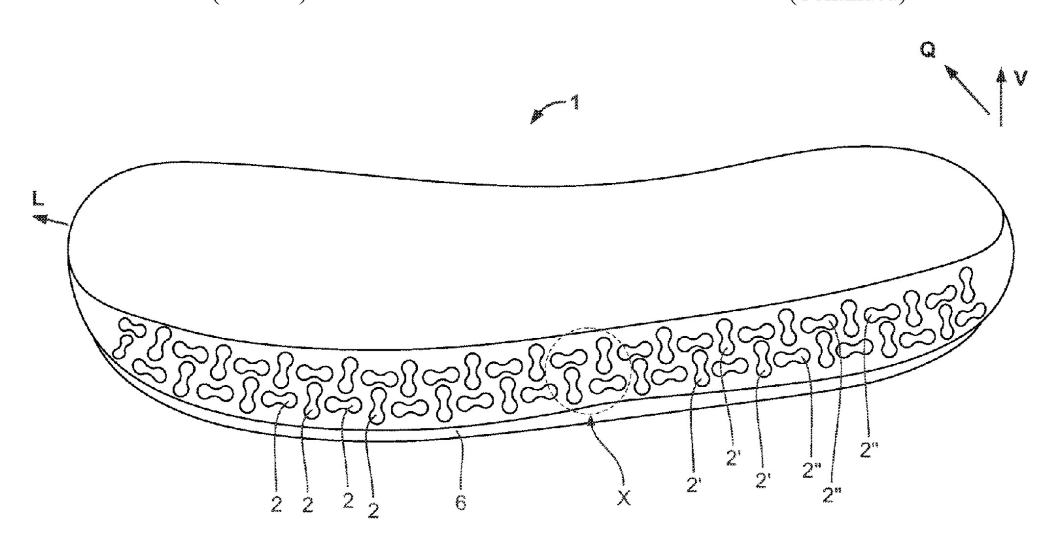
in the longitudinal direction (L), and that there is a second group of recesses (2") which, without external forces on the sole (1), are smaller in the vertical direction (V) than in the longitudinal direction (L), wherein at least in sections, at least one row (3, 4) of recesses (2', 2") is arranged adjacent to each other in the longitudinal direction (L), wherein a recess (2") of the second group is arranged between two recesses (2') of the first group.
