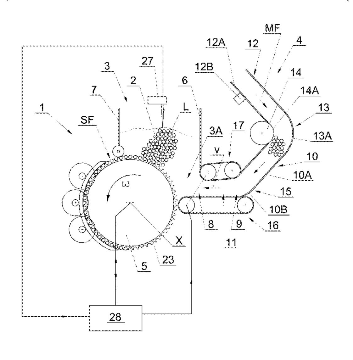
is provided with an upper drive element (17, 33) for the mass flow (MF) comprising a bearing surface (17A, 33A) which is at least partially situated convergently to the bearing surface (16A) of the lower conveyor (16) of the second feeding channel (11) in the direction from the first feeding channel (10) to the storage container (3).
