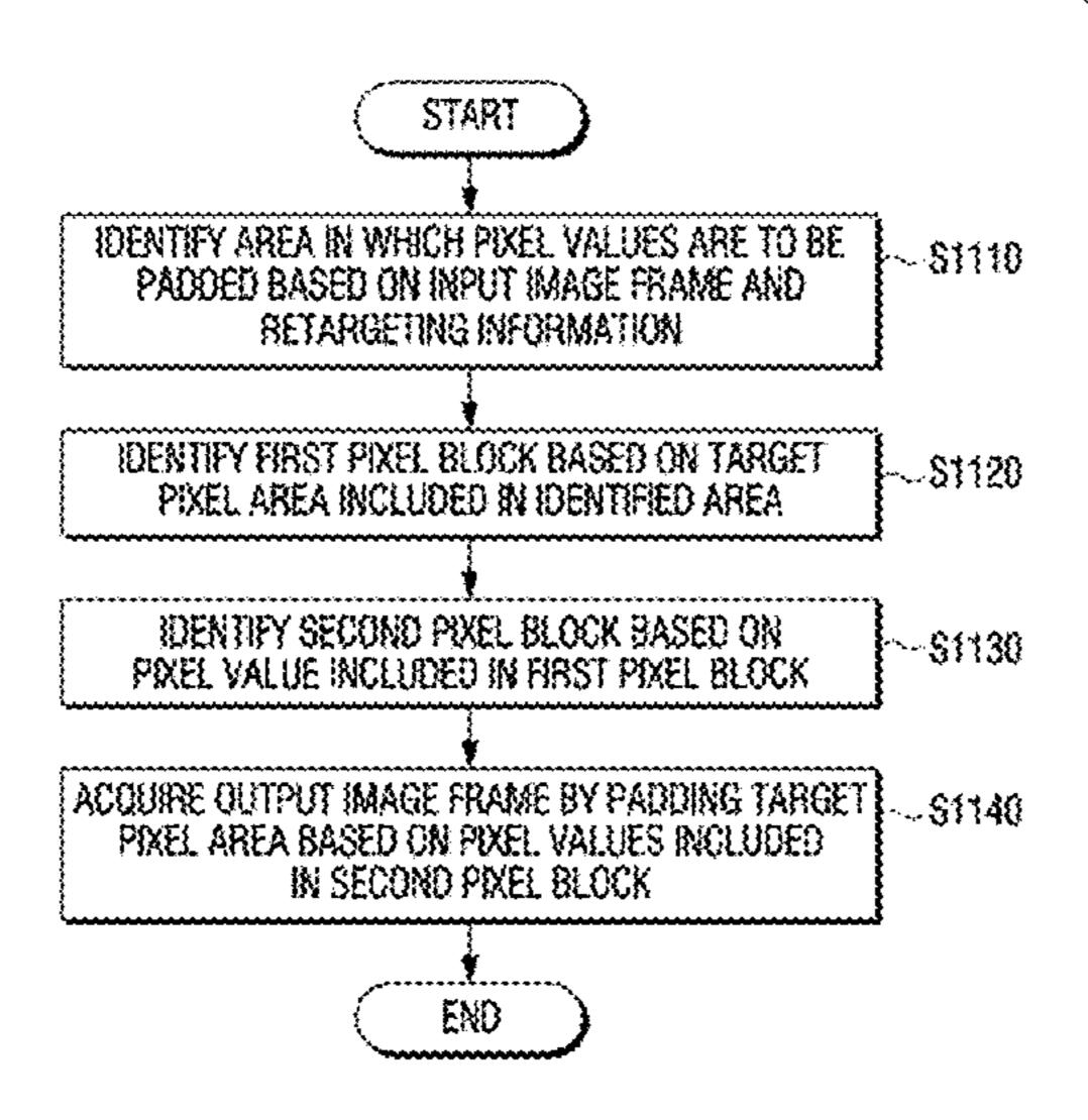
a second pixel block on the basis of pixel values included in the first pixel block, and pads the target pixel area on the basis of pixel values included in the second pixel block, so as to able to acquire the output image frame.
