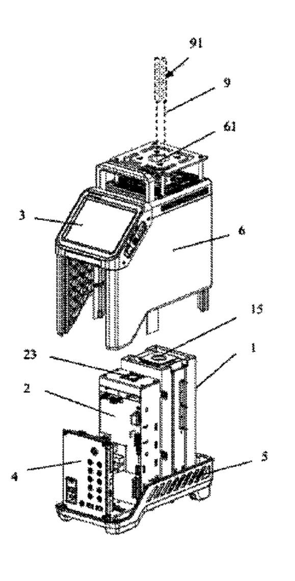
is inserted in the furnace body, such that the handle is cooled, thereby preventing the sensor inside the handle from failing due to high temperature, facilitating the heat dissipation of the internal electronic components of the instrument itself, and extending the service life of the temperature calibrator.
