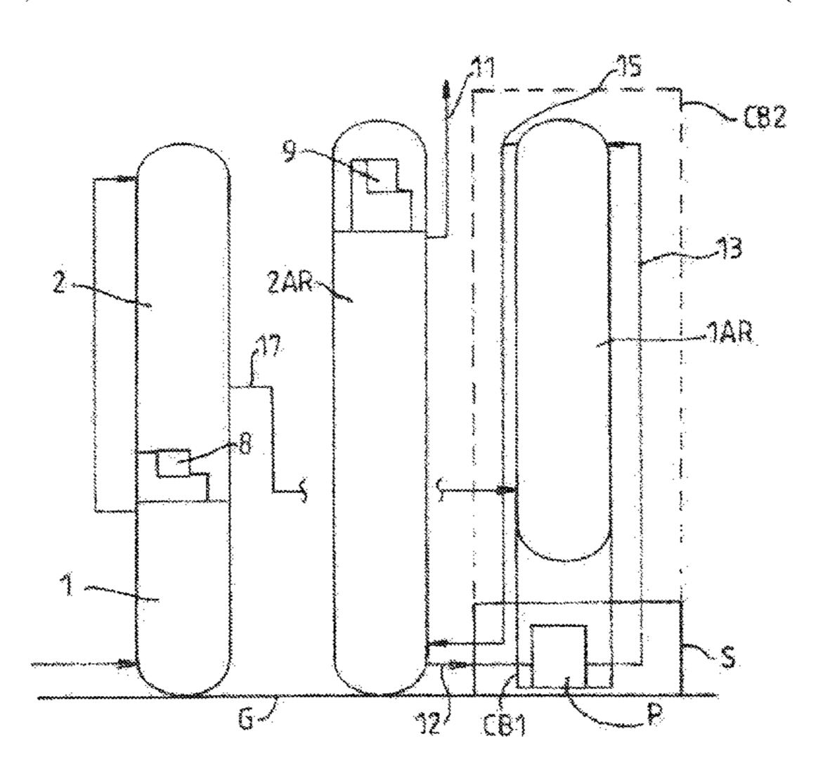
first argon column via the pump, the first end of the first argon column being raised above the ground by a first supporting structure, the pump being positioned within the first supporting structure, such that the pump is at least partially underneath the first end of the first argon column.
