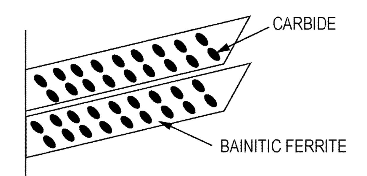
terms of area fraction with respect to the whole steel sheet microstructure, lower bainite in an amount of 40% or more and less than 85%, martensite including tempered martensite in an amount of 5% or more and less than 40%, retained austenite in an amount of 10% or more and 30% or less, and polygonal ferrite in an amount of 10% or less (including 0%).
