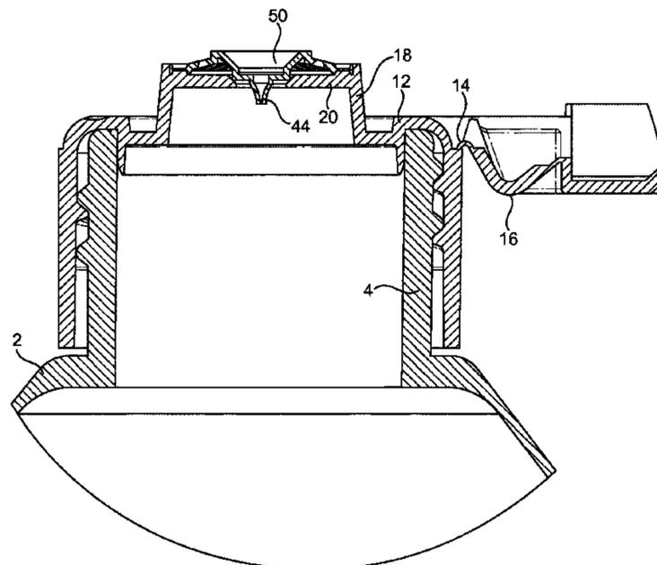
respective opposed annular sealing areas which are situated upstream of the spray slits and are biased into contact with one another by the resilience of the insert. When the spray cap is inverted and an increased pressure is produced in the space the pressure acts on the insert and the insert is thereby caused to deform such that the sealing areas move out of sealing contact and liquid can flow to the spray slits.
