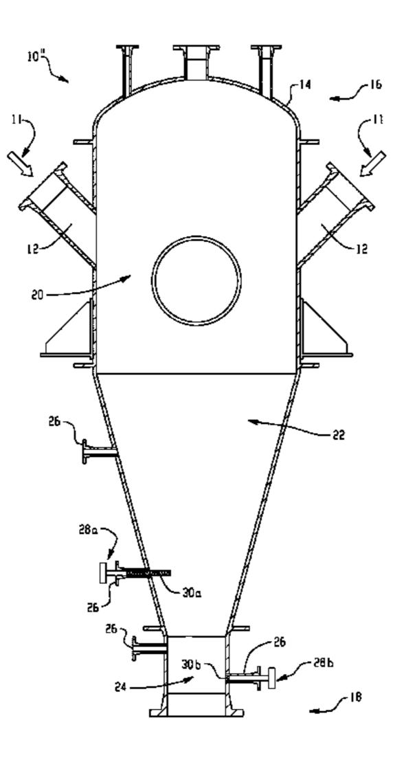
solids from flow 11, and provide for decanting of a liquid layer above the settled solids, and optionally provide for de wetting the settled solids, and provide for discharge of the settled solids (e.g., liquid wetted) from the bottom of the assemblies.
