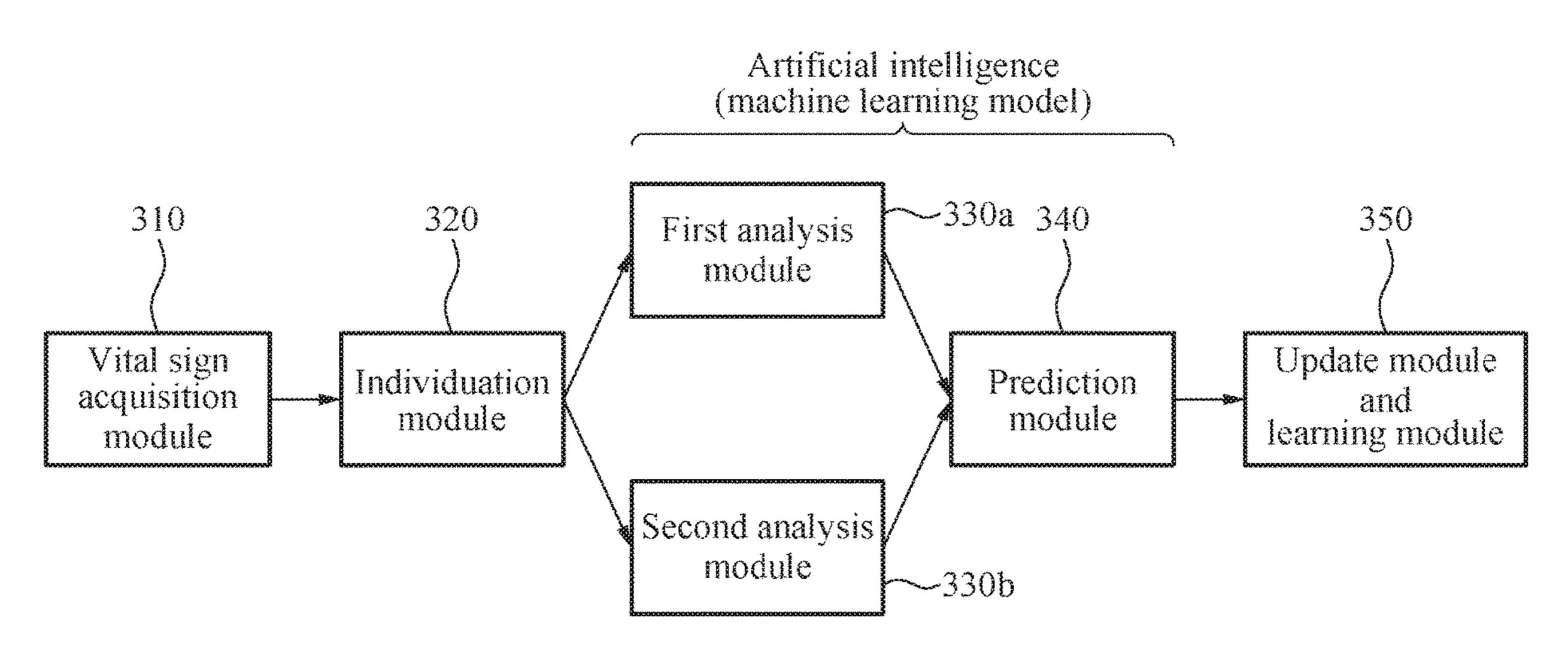
the same into individuated data, generates analysis information from the individuated data on the basis of a machine learning model, generates a prediction result by referring to the analysis information, and provides the prediction result to an external entity.
