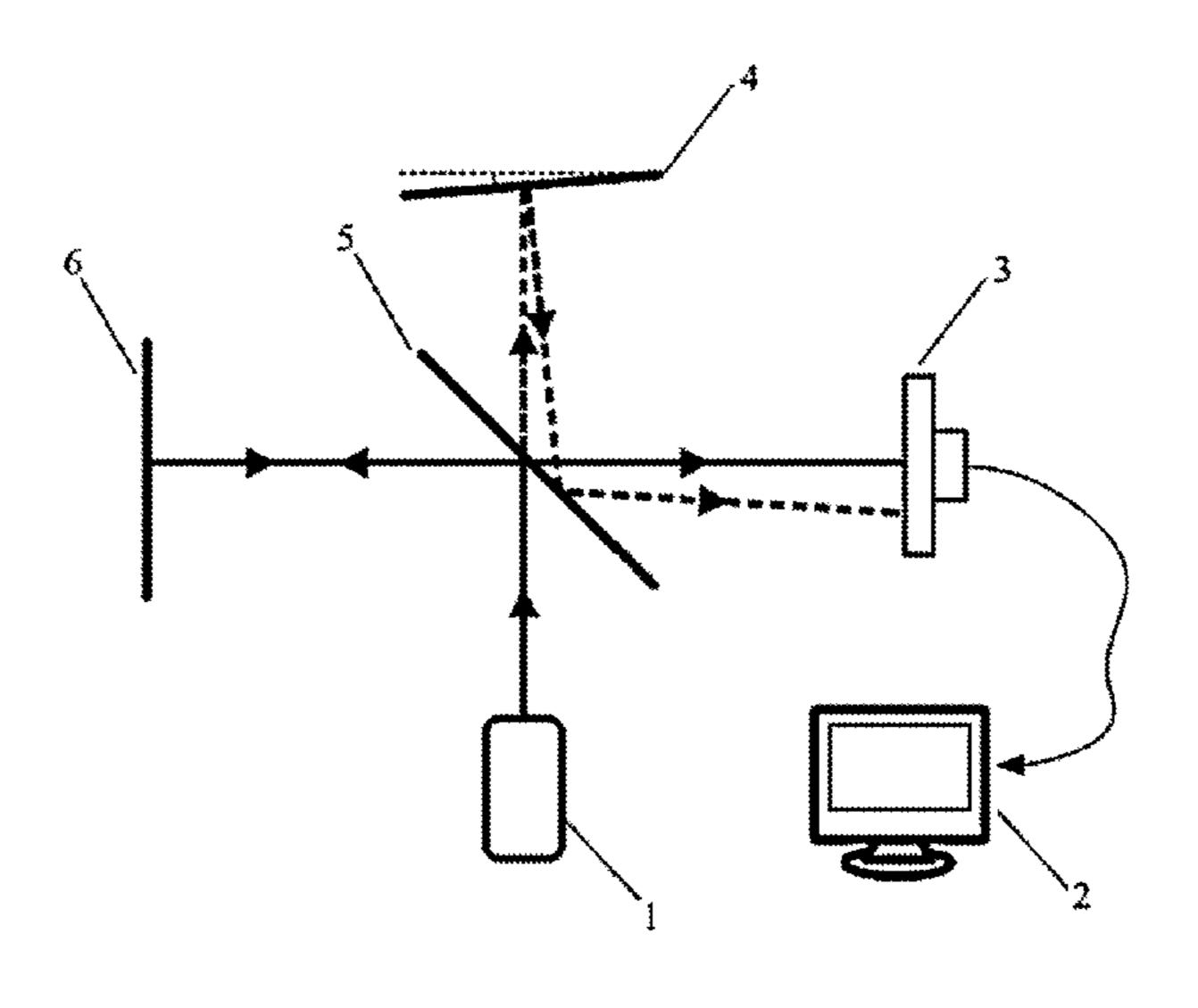
three-degree-of-freedom laser interferometer for displacement and angle measurement is met.
