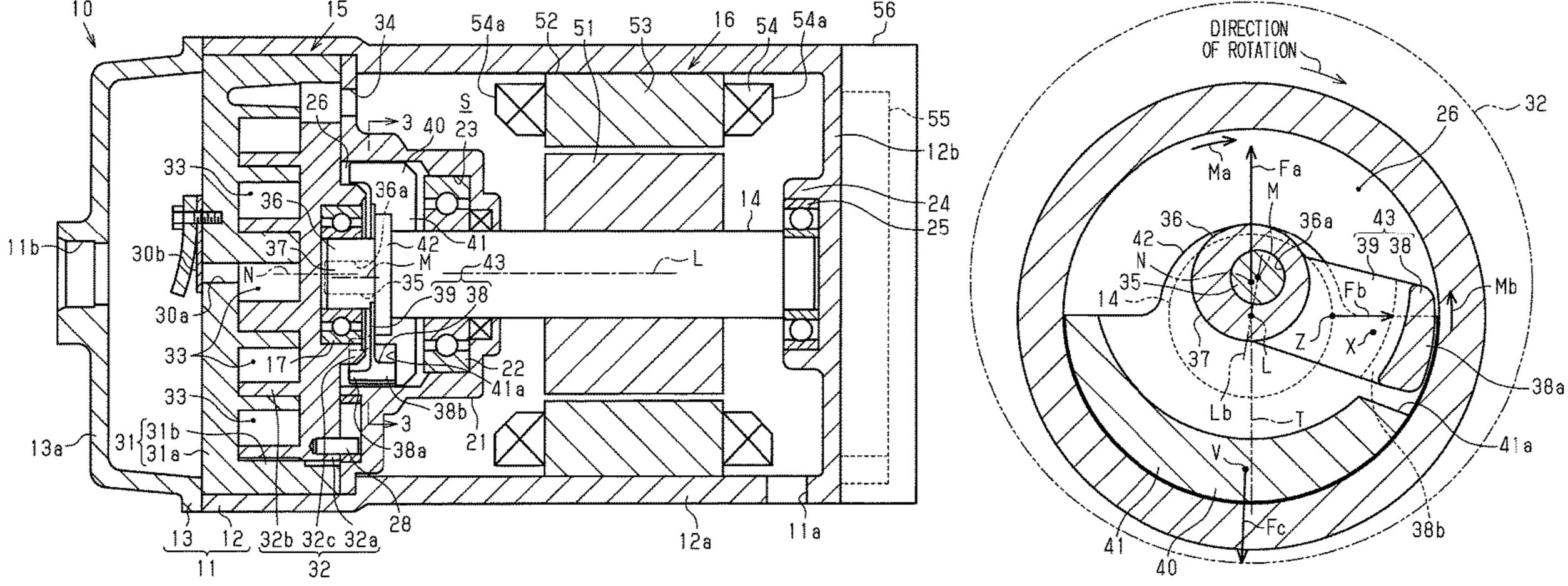
portion due to rotation of the rotary shaft are in the opposite directions. As viewed in the axial direction of the rotary shaft, the center of gravity of the bushing is located on the same side of a straight line including the center of the cylindrical portion and the center of the rotary shaft as the center of the eccentric shaft.
