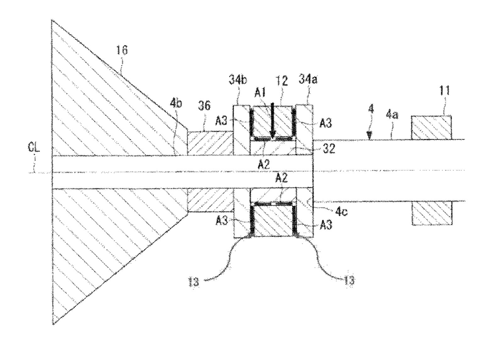
line (CL) direction of the cylindrical sleeve (32), respectively, having a larger diameter than the cylindrical sleeve (32), and configured to rotate together with the rotary shaft (4); and a compressor-side journal bearing (12) arranged on the outer circumference side of the cylindrical sleeve (32) and between the thrust collars (34*a*, 34*b*).
