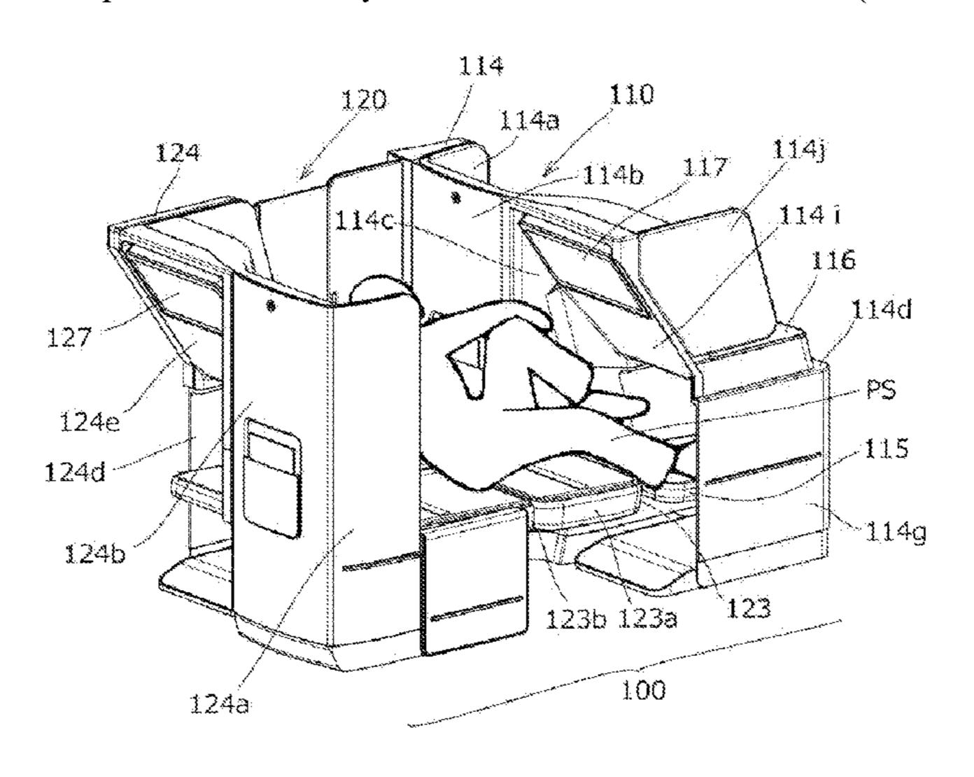
wall, and the partition wall has an inclined surface tilted toward the second seat unit.
