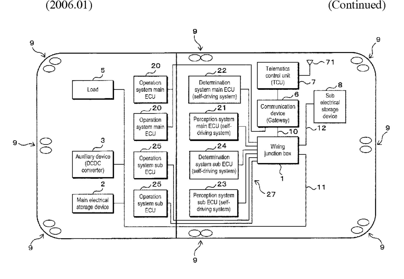
device-side communication port and the ECU-side communication ports, the power line branches according to the number of power output terminals, and the communication line branches according to the number of ECU-side communication ports.
