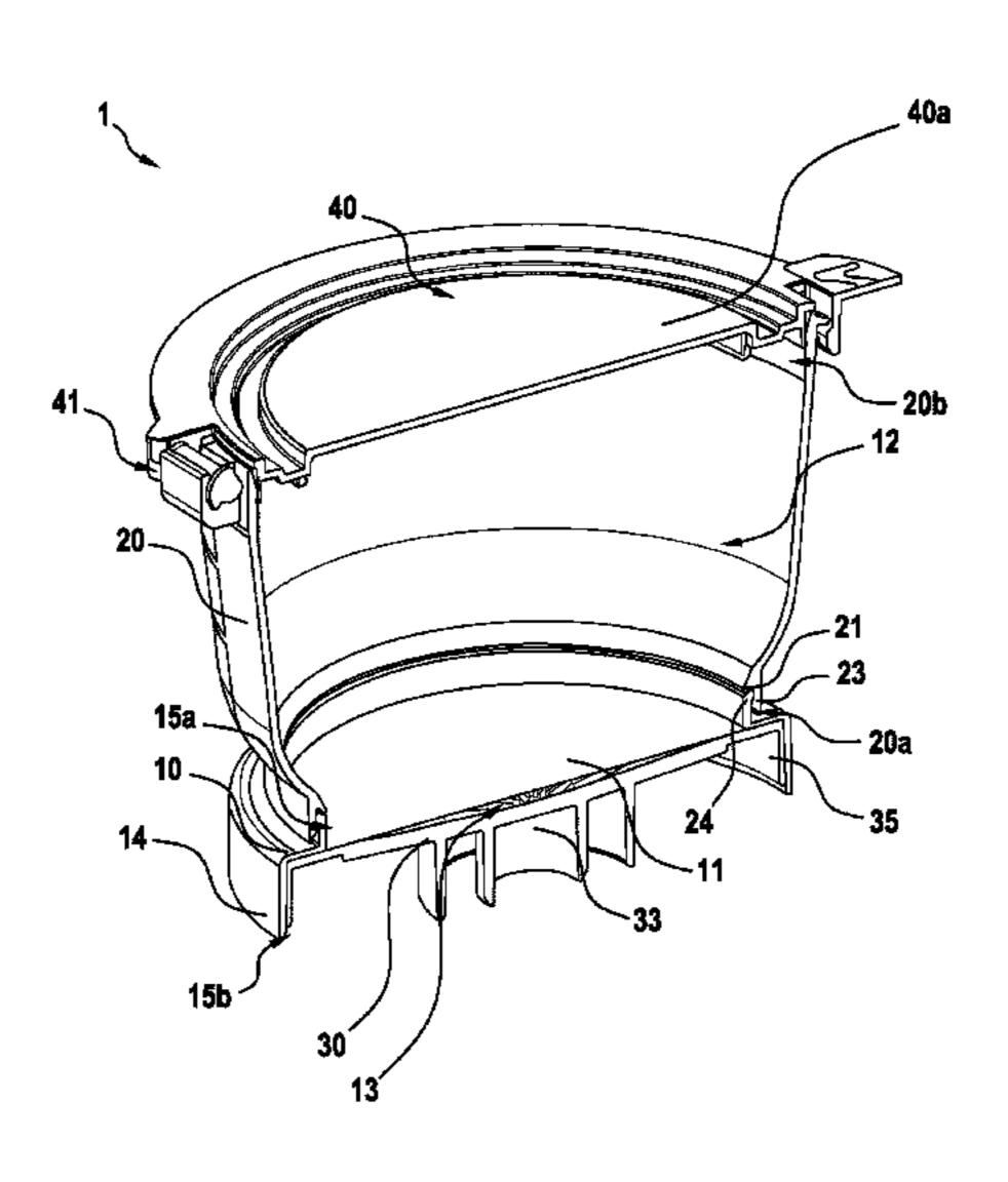
as to seal the one axial side of the membrane support (10) from the environment.
