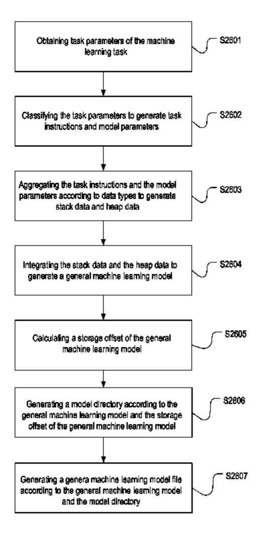
integrating the stack data and the heap data to obtain a general machine learning model (S1204). By means of the method, compiled results of a corresponding general model in the running of an algorithm can be directly executed, which avoids repetitive compilation, thus greatly improving the efficiency of machine learning algorithm implementation and shortening the time from compilation to obtaining execution results.
