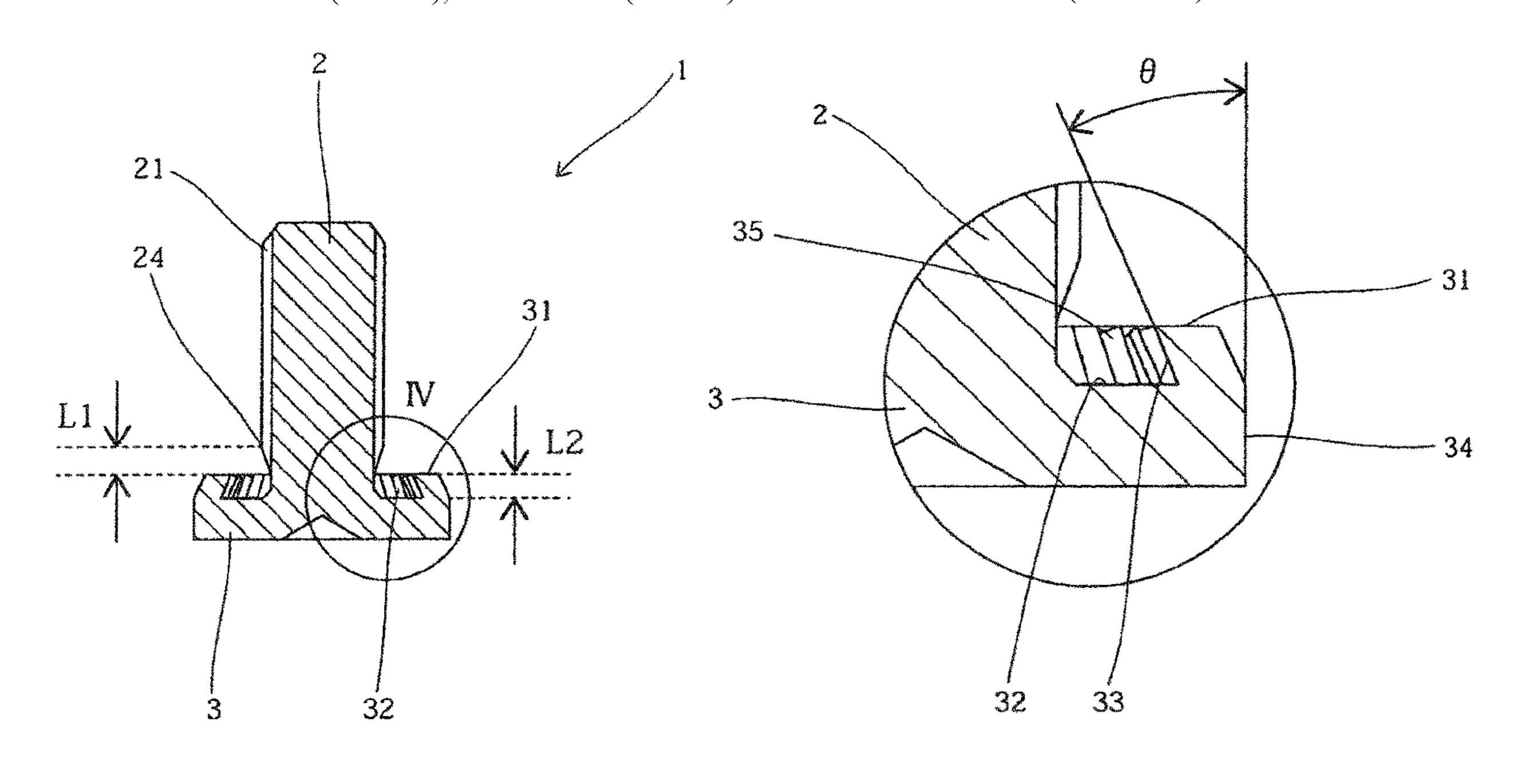
crimped member is fitted. The caulking bolt includes projections and depressions for whirl-stop in the groove.
