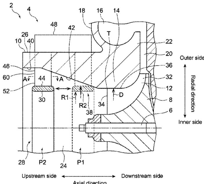
tion configured to move between a first position and a second position upstream of the first position in an axial direction of the impeller, and a strut supporting the annular portion. The strut extends toward at least one of an outer side in a radial direction of the impeller or a downstream side in the axial direction of the impeller with an increase in distance from the annular portion.
