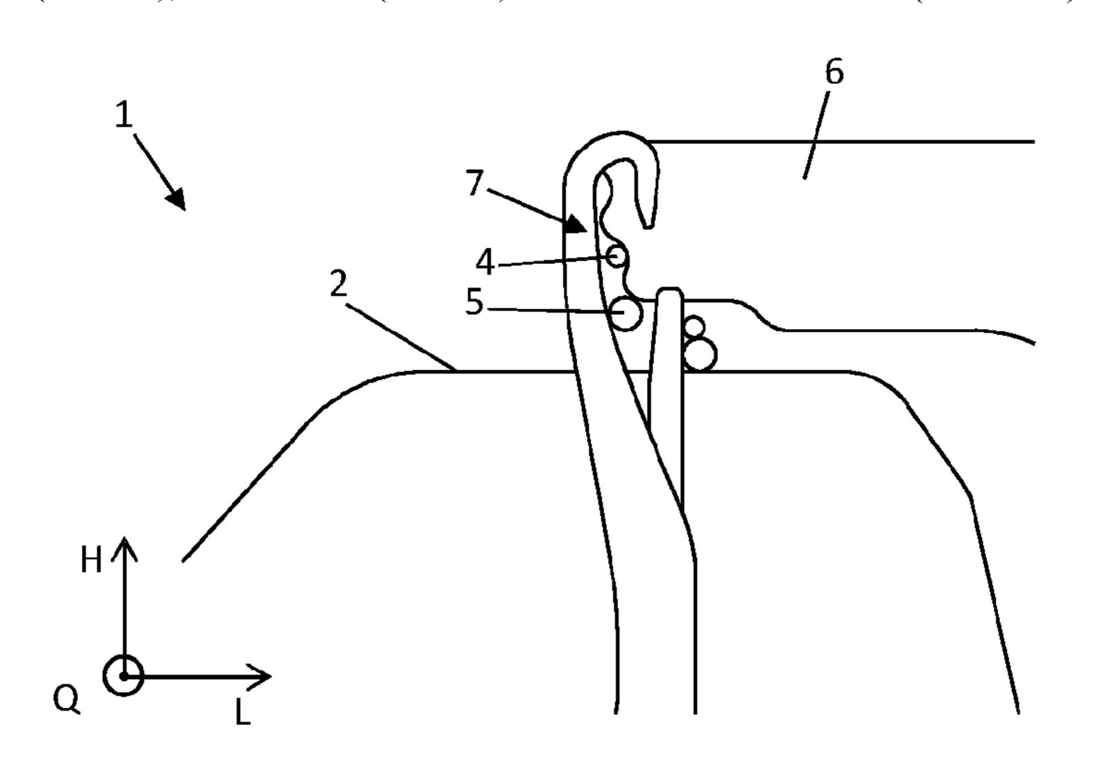
manner relative to the knock-over edge that the guide means performs a movement which, at least section-wise, tracks at least one yarn.
