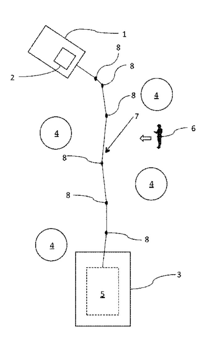
trajectory into the parking slot. Automatically driving the vehicle into the parking slot is repeated multiple times, and involves deleting a feature descriptor stored in the digital map if the number of matches does not exceed a threshold after a predefined number of repetitions.
