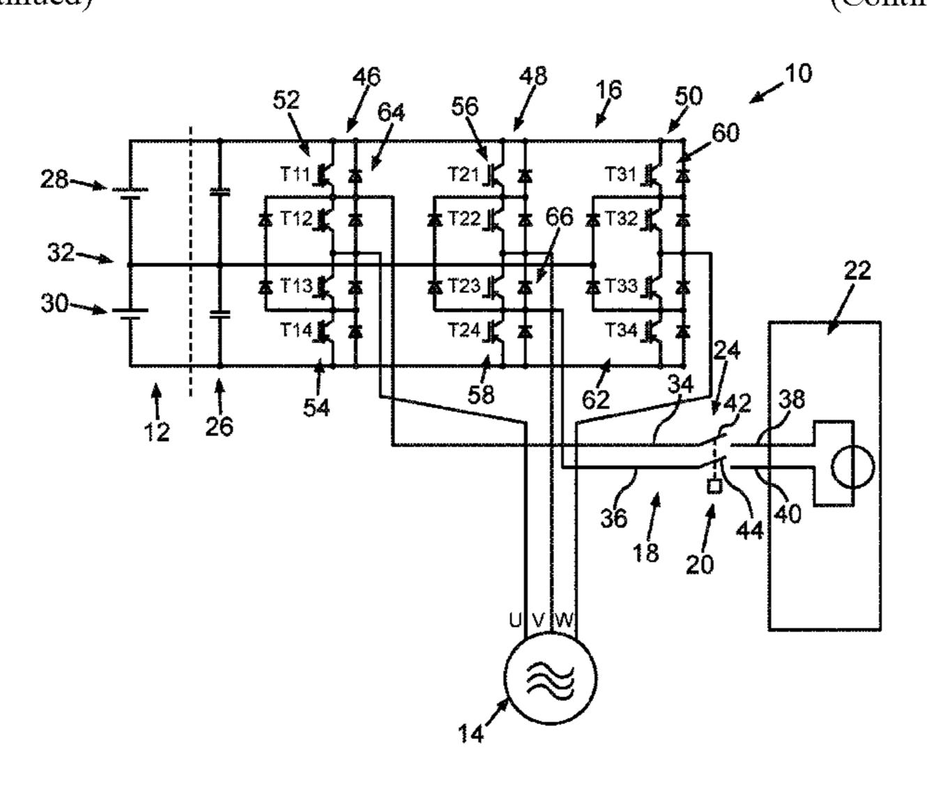
to a first phase of the electric machine. The first switch unit has two switch groups connected in series which each have two insulated-gate bipolar transistors (IGBTs) connected in series, where a connection is disposed between the IGBTs of one of the two switch groups, which connection is electrically connected directly to a line of the charging connection.
