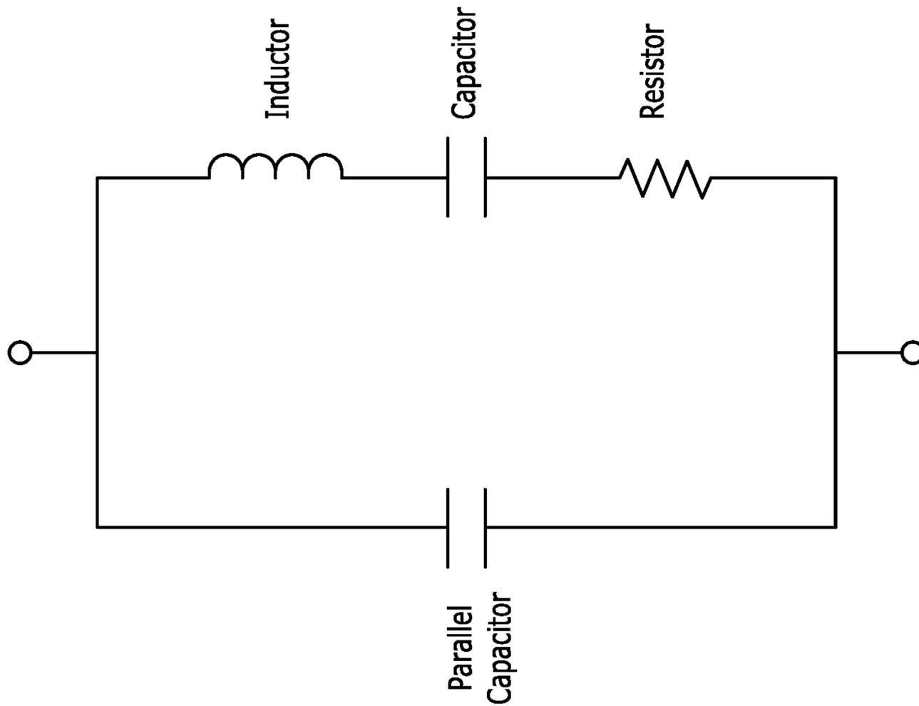
Components of Piezoelectric Transducer in a circuit
