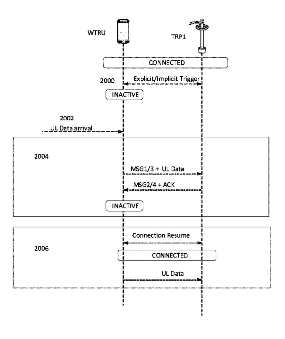
it has moved outside a logical area (e.g., update RAN paging area). Mobility in light connected state may be network controlled (e.g., to enable handover when data transfer may be allowed and/or ongoing). A WTRU may be reachable during a light connectivity state. A WTRU may engage in autonomous mobility during light connectivity and/or an Inactive state.
