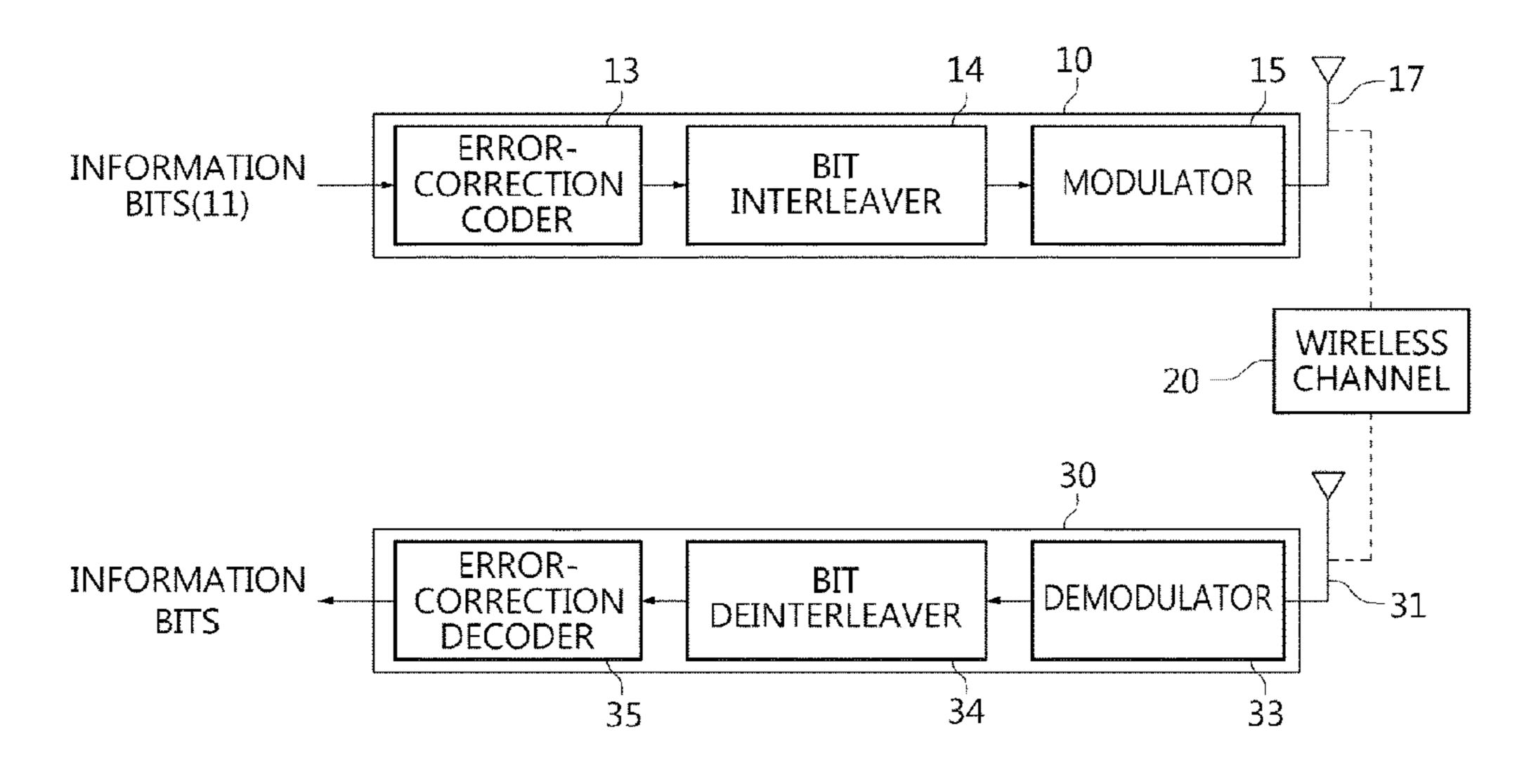
of 16200 and a code rate of 4/15. The processor generates an interleaved codeword by interleaving the LDPC codeword on a bit group basis. The size of the bit group corresponds to a parallel factor of the LDPC codeword. The second memory provides the interleaved codeword to a modulator for 16-symbol mapping.
