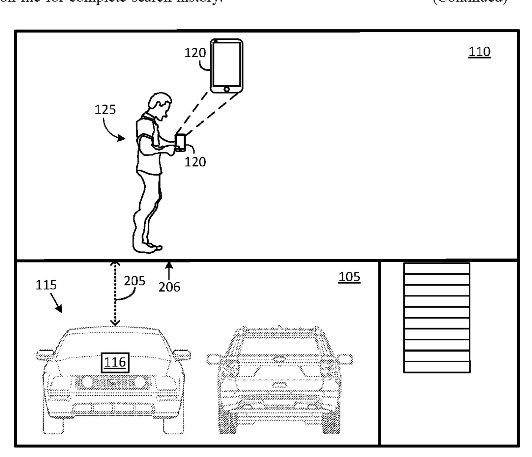
detect a presence of a mobile device (such as a phone-asa-key or a vehicle key fob) and determines the location of the mobile device based on the dimensional information. If the mobile device is located outside the garage, the vehicle entry authorization system refrains from activating a component of the vehicle. However, if the mobile device is located inside the garage, the vehicle entry authorization system activates the component.
