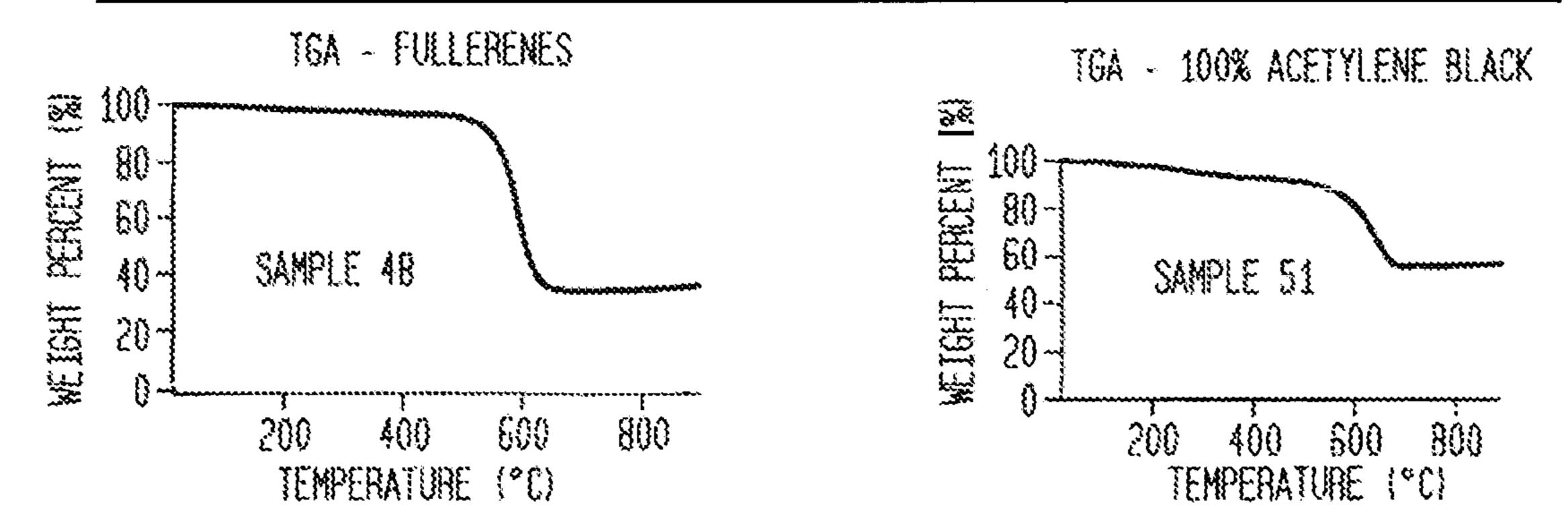
CONDUCTED UNDER THE FOLLOWING CONDITIONS: BALANCE GAS: NITROGEN 40.0 ml/min. SAMPLE GAS: AIR 60.0 ml/min. RAMP 20.00° C/min TO 900° C
