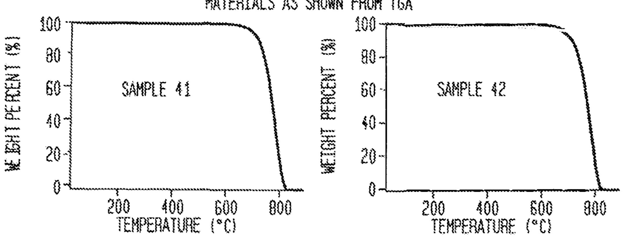
CONDUCTED UNDER THE FOLLOWING CONDITIONS: BALANCE GAS: NITROSEN 40.0 ml/min; SAMPLE GAS: AIR 60.0 ml/min; RAMP 20.00° C/min TO 900° C
