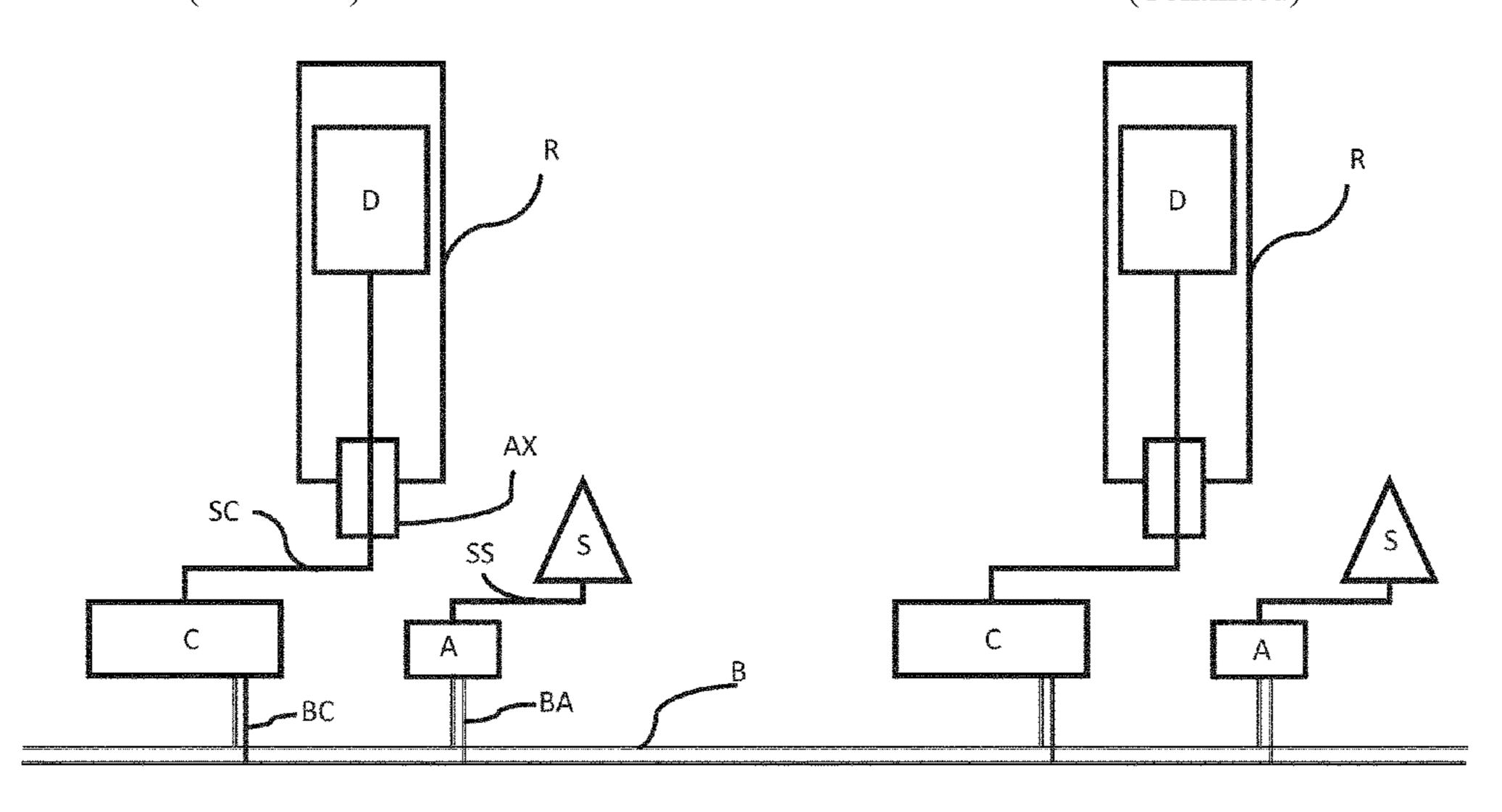
sensor signal data block which characterises the sensor signal and a sensor address data block, and to transmit the bus-encoded sensor data block into the bus line.
