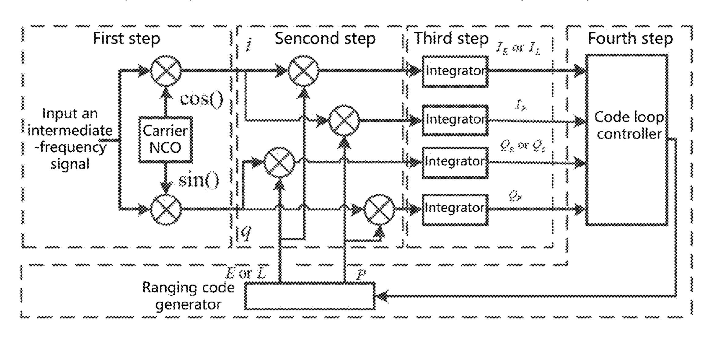
steepest descent method, such that the loop has a multipath suppression function without increasing the computational burden. Compared with a narrow-distance correlation method, the current method reduces computing resources by ½, the design and adjustment of parameters are simple and feasible, a multipath suppression effect is superior, and a high engineering application value is obtained.
