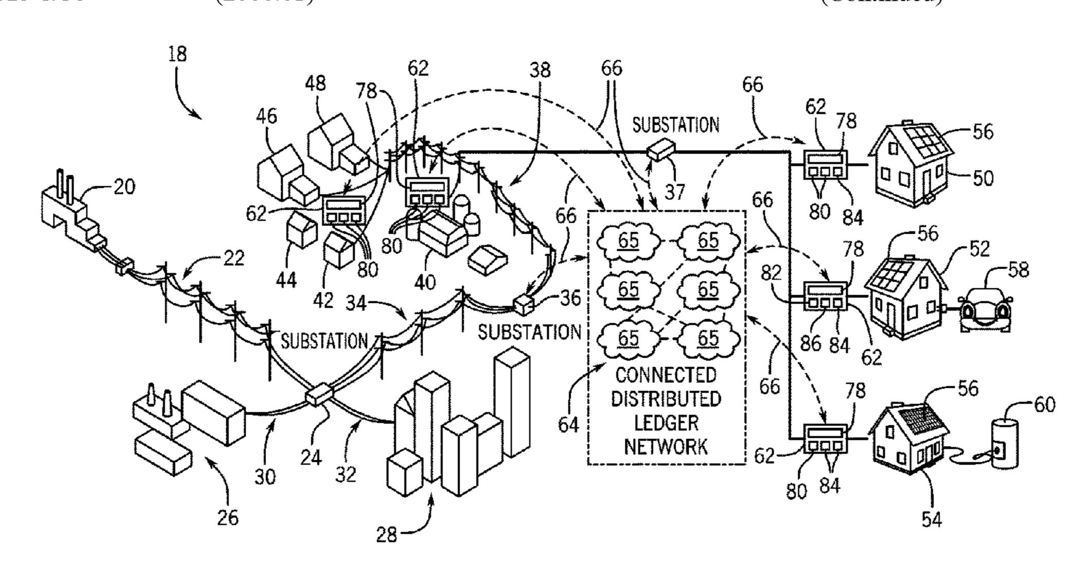
one of supply of electricity from one of a plurality of available energy sources to an on-site load based on predetermined demand parameters set by an energy buyer and delivery of electricity generated by a distributed energy resource to an external load based on predetermined supply parameters set by an energy supplier.
