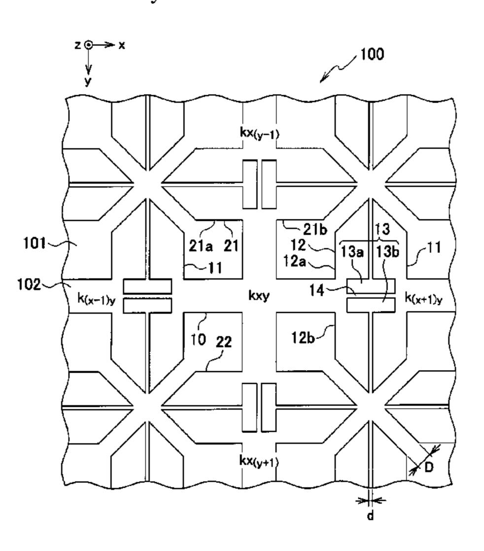
interval of the tip portion is wider than an interval with the electrode plate part of the other adjacent resonator.
