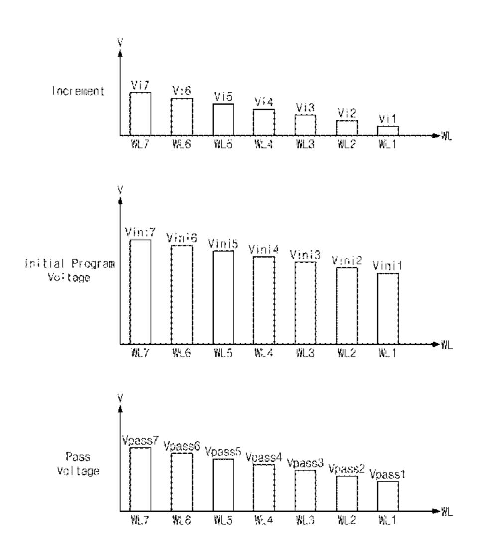
nitudes of the word line voltages may be determined according to locations of the plurality of word lines.
