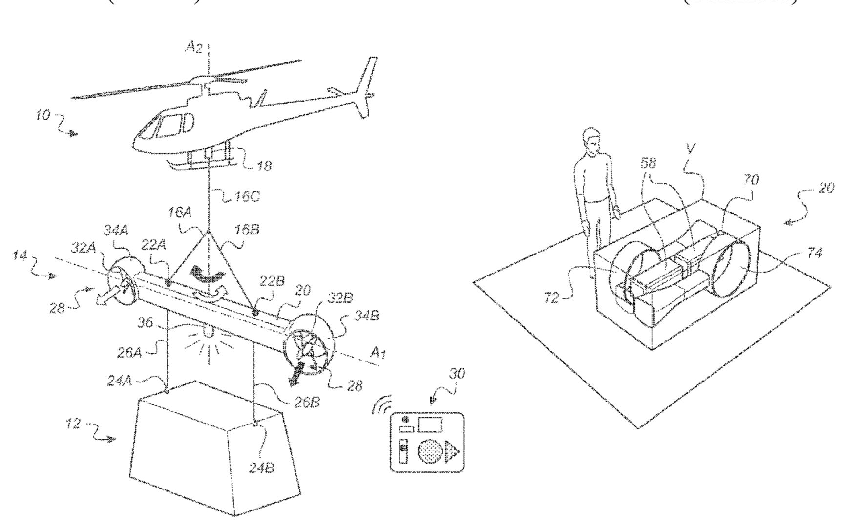
the spreader beam about its vertical transverse axis. The spreader beam includes a propulsion unig disposed in such a way as to engage its rotation, selectively in one direction or in the other, about its vertical transverse axis when it is suspended from the machine via the sling system.
