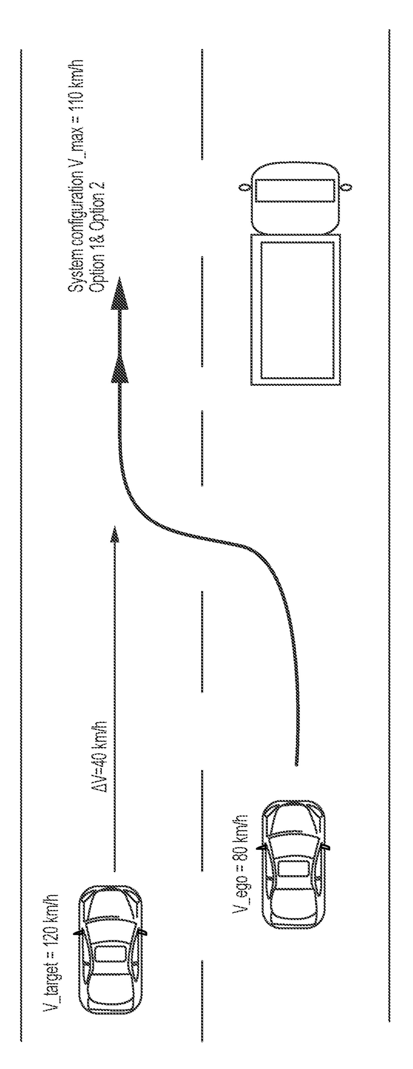
Option 1: Accelerate to adapt with V\_target and execute lane change fully automatically Option 1: Driver is able to trigger the lane change maneuver Option 1a: Driver is able to trigger the lane change maneuver Option 2: Display V\_target proposal to driver -> manual acceleration and manual lane change.
