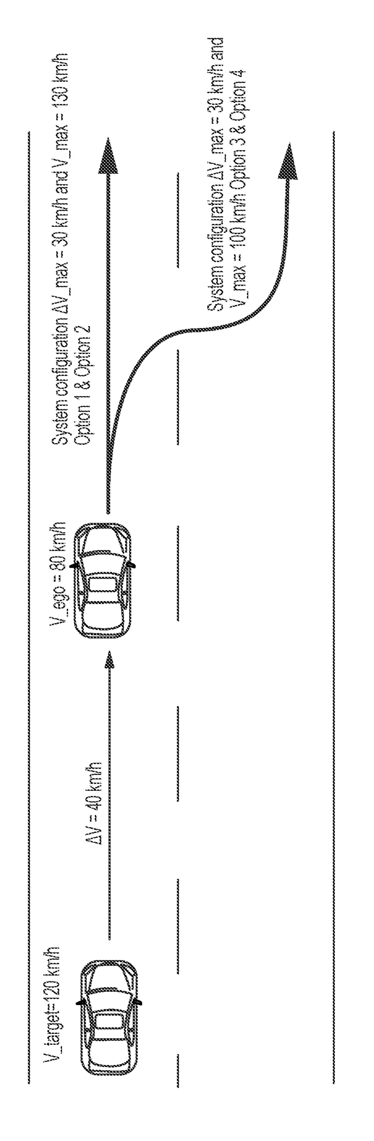
Option 1: Accelerate automatically to adapt with V\_target Option 2: Display V\_target proposal to driver ->manual acceleration
