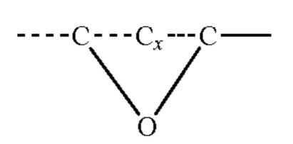
wherein x is zero or a whole number, typically from 1 to 4. Other potential epoxy resins typically used in foundry
