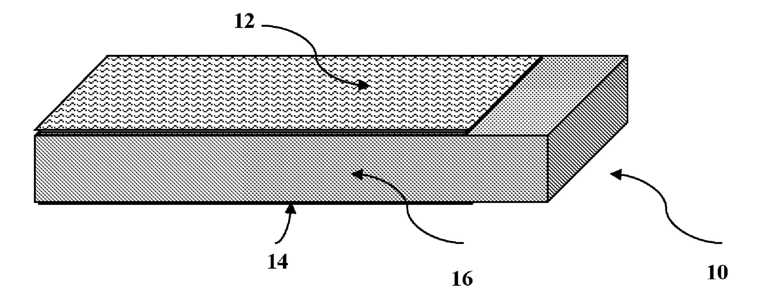
reinforcement can be formed from a woven or non-woven material, such as glass fibers. The composite panel can further include a material, such as a second fiber reinforcement and a cementitious layer, in contact with the second surface of the polyurethane composite. Articles comprising the composite panels are also disclosed.
