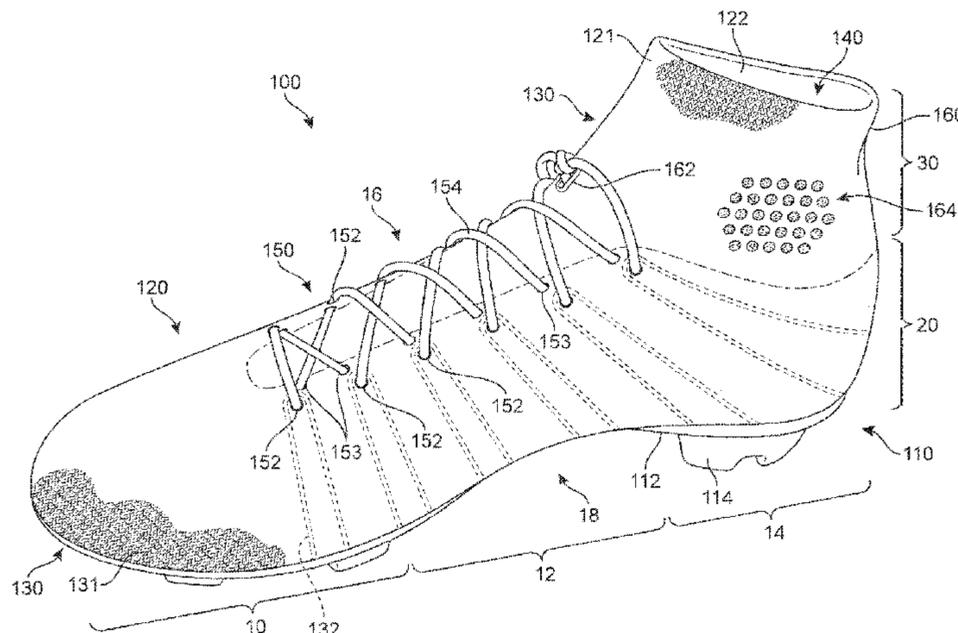
orientation of the upper of the article of footwear when being worn.
