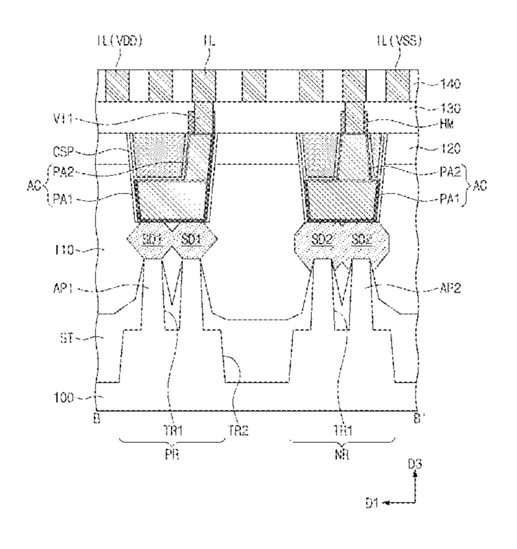
contact hole and a second segment that vertically protrudes from the first segment. The first via is connected to the second segment. The insulating pattern is adjacent in the first direction to the second via.
