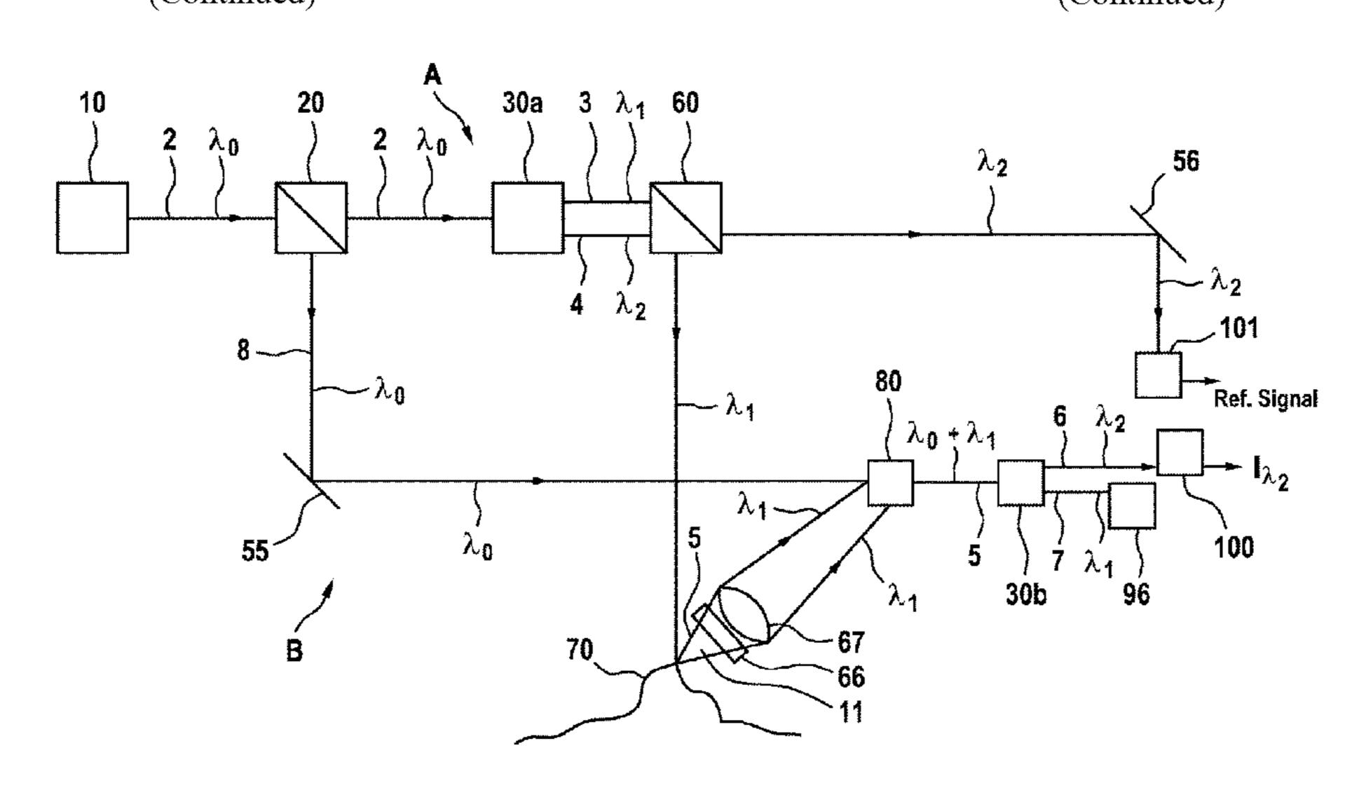
frequency, and a detection-signal being generated so that the object-distance is determinable due to the aforementioned superposition based on the time-difference between the detection of the first light-beam including the reference-frequency and a detection of a change of the reference-beam including the reference-frequency.
