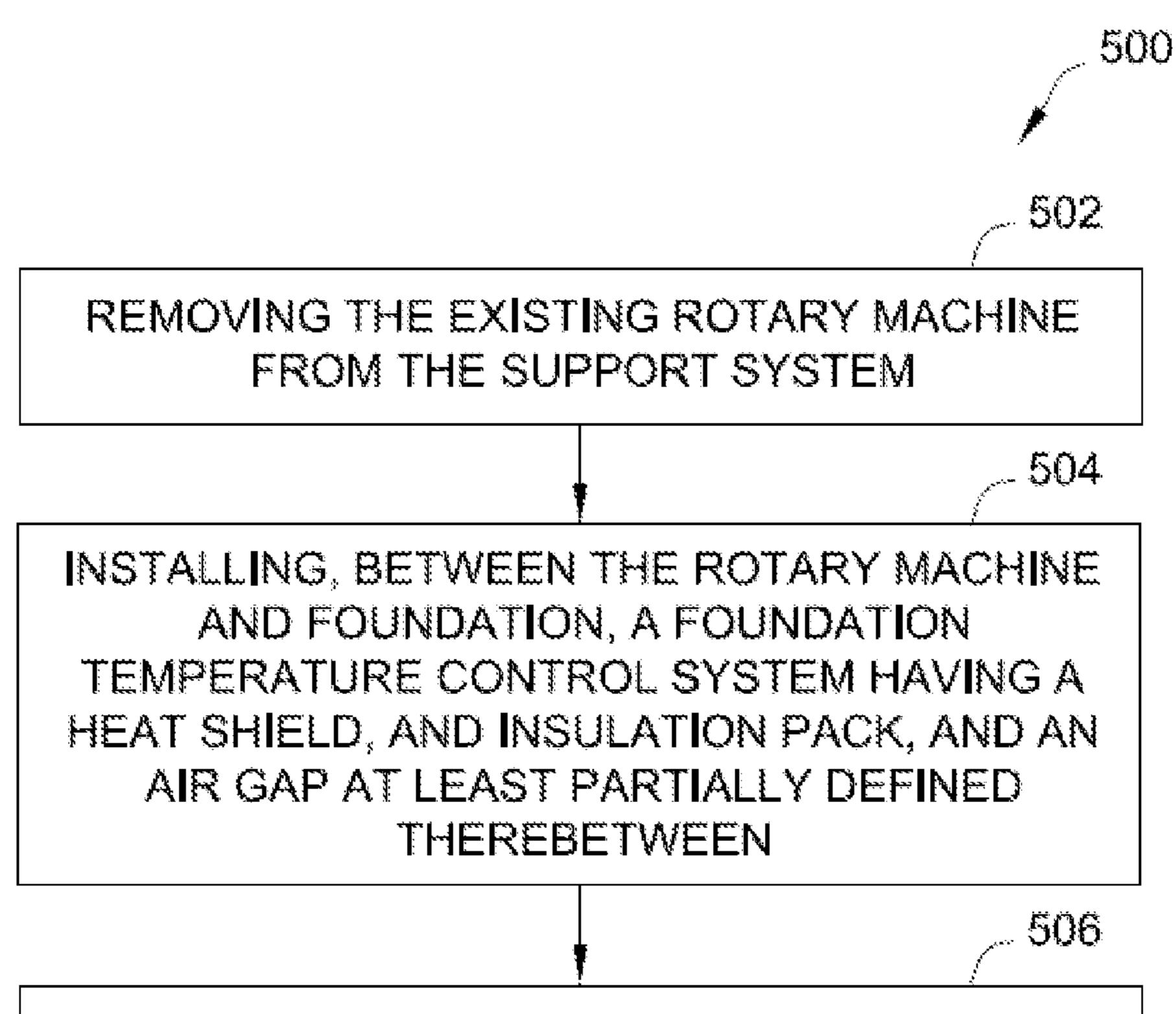
INSTALLING THE NEW ROTARY MACHINE ON THE SUPPORT SYSTEM, SUCH THAT THE FOUNDATION TEMPERATURE CONTROL SYSTEM IS BETWEEN THE NEW ROTARY MACHINE AND THE FOUNDATION, WHEREBY, DURING OPERATION OF THE NEW ROTARY MACHINE, HEAT IS RADIATED TOWARDS THE FOUNDATION, AND THE HEAT SHIELD, THE INSULATION PACK, AND THE AIR GAP MAINTAIN A TEMPERATURE OF THE FOUNDATION BELOW A MAXIMUM RATED OPERATING TEMPERATURE OF THE FOUNDATION
