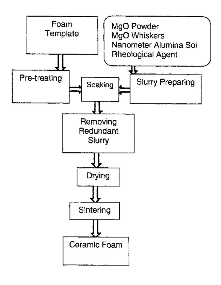
drying the biscuit by heating it to 80° C.-1200° C.; 3) putting the dried biscuit into a sintering furnace, elevating the temperature to 1400° C.-1600° C. and performing a high temperature sintering, cooling to the room temperature with the furnace to obtain the magnesium oxide-based ceramic foam filter.
