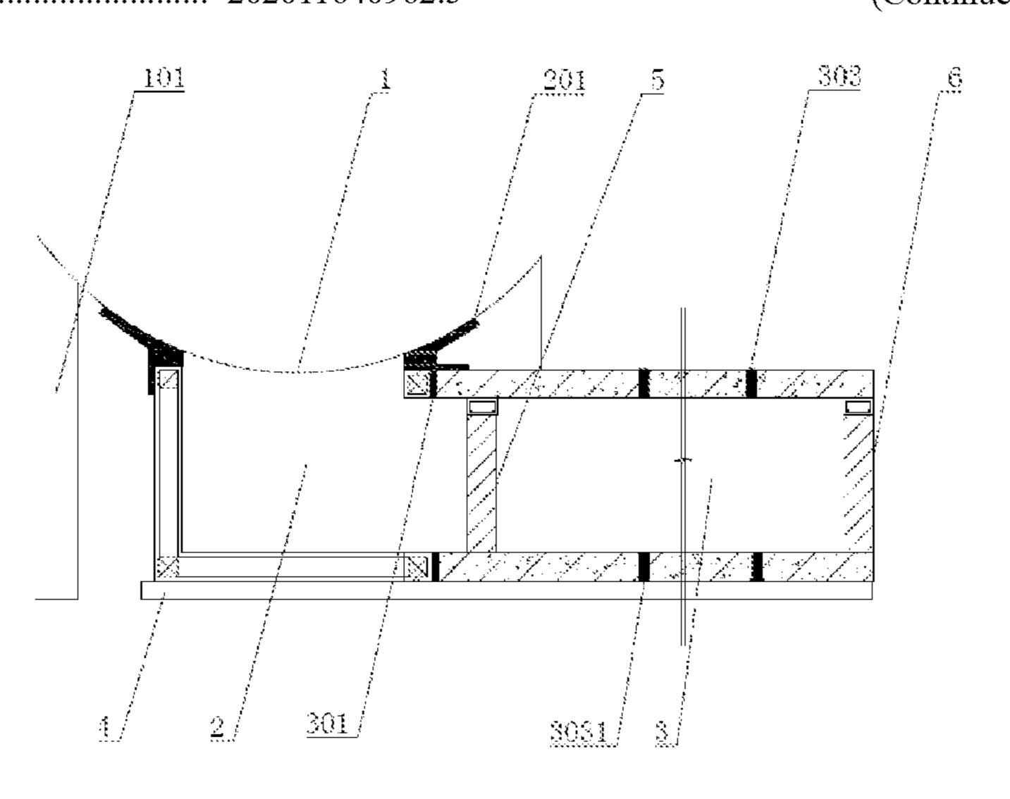
covered with soil, and the spherical tank body is supported by a stand column and is arranged on the ground, such that a gap is formed between the bottom of the spherical tank body and a ground foundation; the valve chamber is arranged between the spherical tank body and the ground foundation; a top opening of the valve chamber is connected to the bottom of the spherical tank body by means of a first connecting structure.
